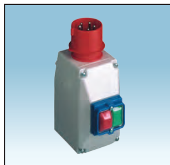
Insulated enclosure with CEE-plug IP 54 16 A, 5-pole, 3P + N + PE 1 opening at the bottom
